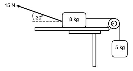
The coefficient of kinetic friction between the 8 kg block and the surface of the table is 0,25. Ignore the effects of air friction.
