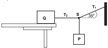
The tension in the string connecting block  $\mathbf{Q}$  is  $T_2$  and that for the string that pulls at  $35^{\circ}$  is  $T_1$  as shown in the diagram.
