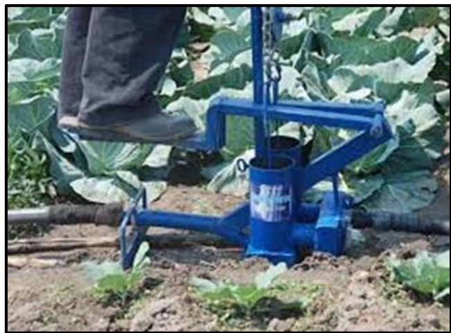
Easy to use tread pump can pump water from a well or a river and easily transported.
